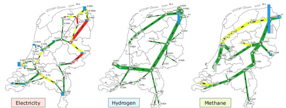
Figure 7: Intensity representation of a flow pattern for a typical snapshot (green = moderate loading; yellow = high loading; red = overloaded; line width proportional to flow)
